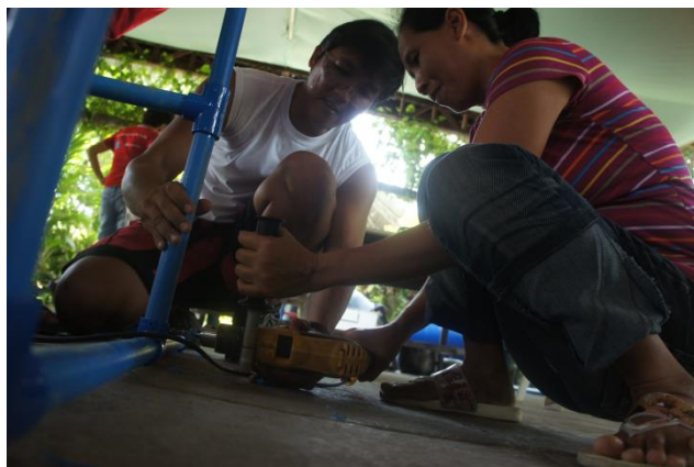
Figure 17. Top photo shows the author teaching a woman volunteer use the electric drill to bore holes into the PVC pipes of the dryer during the skills training on June 2014. The training was part of the campaign of the Save the Children to create
