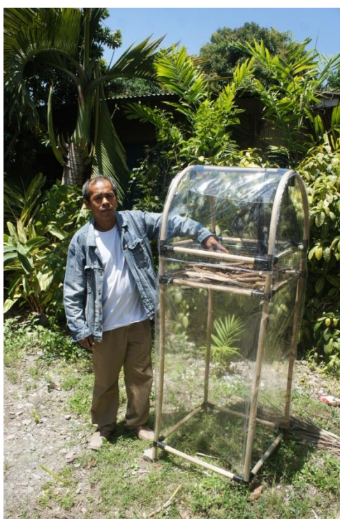
Figure 16. The solar dryer tower as it was being tested in the City of Danao (left photo). It was built with rattan poles that were fixed with metal connectors (top photo). The lower two thirds section of the dryer serves as the hot air generator while the upper one third serves as the drying section.
