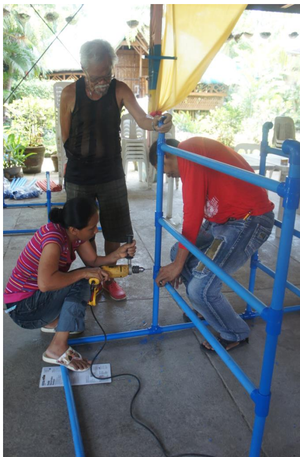
Figure 17. Top photo shows the author teaching a woman volunteer use the electric drill to bore holes into the PVC pipes of the dryer during the skills training on June 2014. The training was part of the campaign of the Save the Children to create
