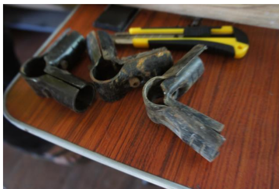
Figure 16. The solar dryer tower as it was being tested in the City of Danao (left photo). It was built with rattan poles that were fixed with metal connectors (top photo). The lower two thirds section of the dryer serves as the hot air generator while the upper one third serves as the drying section.
